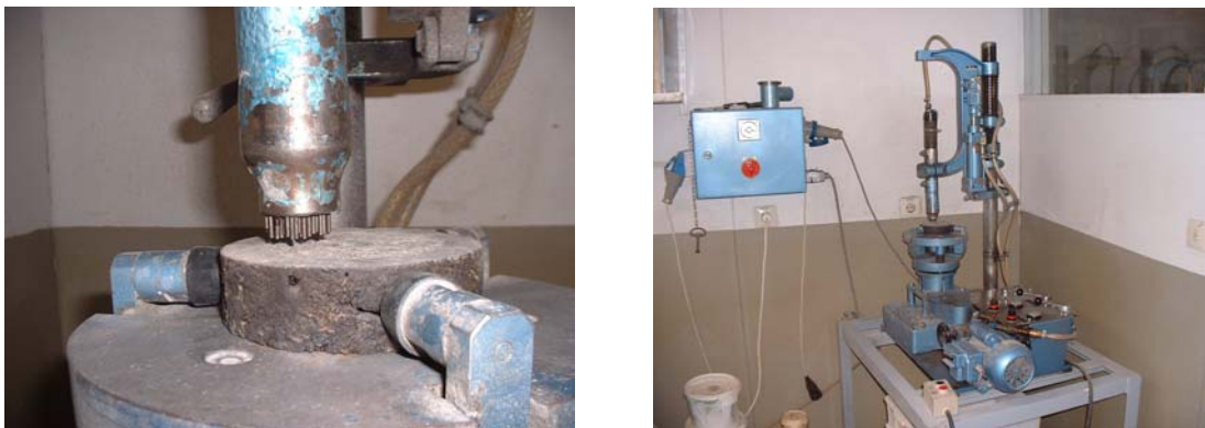
Figure 11. Equipment for measuring resistance of asphalt to studded tyres (Tröger Instruments) used in this study to collect asphalt PM.
