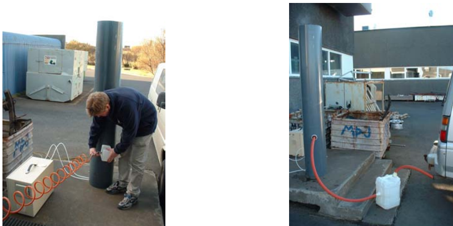
Figure 10. Collection of source samples. Diesel and gasoline collection is shown to the right and soil, brake lining and salt to the left.
